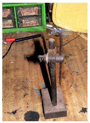
I use this scriber when I'm turning wood to mark where I want to put the next raised part or hollow part in the rod that I'm turning down. It's a marker with a heavy base that sits on the bench and lets you know exactly where to put the next cut in without having to scrawl all over the job.
