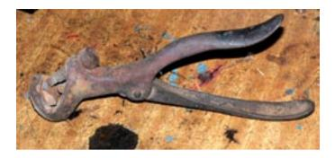
A saw-set. I've got three or four of those. You put it over the tooth of the saw and held it horizontal and when you squeezed it a little piece of metal bent the tooth over to set it so that it wouldn't bind in the cut. It pushed the tooth away from you, so you did every second tooth on one side, then turned the saw around to set every second tooth on the other.
