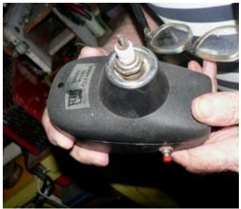
This is a spark plug cleaner. It works off a 12 volt battery. There's a little switch there to switch it on and off. You put the plug into a sort of rubber grommet. There's a little fan inside that activates a shower of small particles of carborundum type of thing and they blow around inside and in a couple of seconds the spark plug comes out shiny bright and clean.
