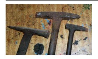
Various hammers for splitting or breaking up rocks and so on.
