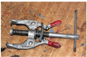
This is a puller specially for removing the battery clips from battery terminals. Sometimes the clips are buggers to get off the terminals, and with this you can pull them off without damaging the terminal.
