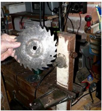
I made this gadget myself. It has provision for sharpening two circular saws. The spindle on the top takes a seven inch saw blade, and the one on the bottom is for a nine and a quarter inch saw blade.
