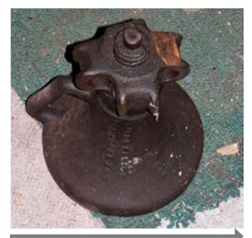
This little mechanism was used for splitting nuts. This would have been used on a nut that was on about a half inch bolt or threaded rod. If the bolt was rusted on or you couldn't undo it without damaging the bolt, then this was used to split the nut. You simply fitted it over the nut, and by screwing the little thing on the right you pushed a little pusher forward and it split the nut.
