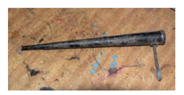
A blowpipe. It was used in the chemistry lab. You'd have your Bunsen burner going, and if you wanted to heat up a crystal or something to break it you put the small end of the pipe near the flame and you blew into the other end, and that directed the flame onto the piece that you wanted heat up.
