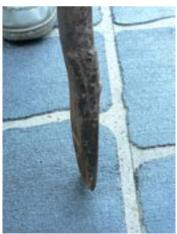
Here's a spud bar, or crowbar, made out of the tailshaft of a 1926 T-Model Ford. These splines at the top engaged with the engine and the shaft reached back to the differential. It was made into a spud bar in a blacksmith's forge. It'll never bend. A bloke wanted to buy it from me but while I'm alive I'm not selling it.
