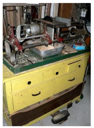
I made this cabinet myself. On top of it is the Sher Shopmate, which can be used as a sawbench, it can be used for vertical drilling, or it can be used as a lathe. A very useful tool. And I made the cupboard, there, where I keep the different parts of the different tools that I use with it. Down the bottom you can see the foot-operated control that I made for it from a converted foot pedal from a Singer sewing machine. It's adjustable speed – the more you push down on it the faster it goes.
