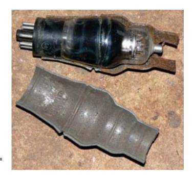
screen was put in as well, and so then we had a valve which was (from the inside) the hot filament, then the cathode, then the grid, then the screen, then the suppressor grid, then finally we had the plate. That was the ordinary efficient valve of the 1930s, 40, and 50s.
