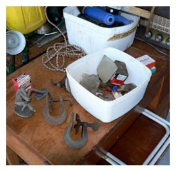
These are vulcanising patches. You used to use them to patch car inner tubes. When you got a puncture you'd scour the spot around the puncture, clamp a special rubber patch over it with these special clamps, then light it, and it would smoulder and fizz away and vulcanise the patch on to the inner tube.
