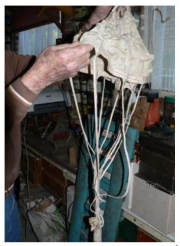
Here is a parachute off the ejector seat of a Sabre aircraft. When you ejected, the seat shot out with the pilot sitting in it. Then he released the seat, and so the seat didn't fall on top of anybody, the parachute let it down gently.
