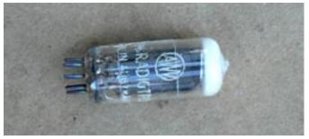
This is a little valve that came out during the war and was used for about twenty years or so. I just included this one because it shows an area of white at the top, which means that air has got into the valve and it is no longer a vacuum – and a vacuum is essential for the working of all valves
