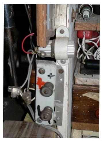
I made this little gadget recently - just two terminals, to connect the battery which is down underneath the bench up to waist high where I have a socket for a cigarette lighter. It gives me a positive and negative terminal and I don't have to go down to the battery underneath the bench if I want to put a couple of bulldog clips on it to make something work, such as the spark plug cleaner.
