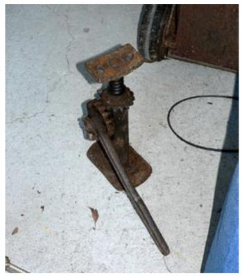
This jack is from a T-Model Ford one-ton truck. It goes with that spanner we talked about earlier and the tailshaft/crowbar. I had that truck when I was working for the PMG in the 1930s.
