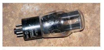
Here we have an Octel valve – that is, a valve with eight pins on the socket at the bottom and a central rod with a keyway on it which would only allow the valve to be inserted in a certain direction. This valve is surrounded by a metal shield which was not only for when the valve was working well, but it was also emitting radio frequency waves which could be picked up by other valves nearby. This meant that it had to be shielded by a metal shield that went around the valve.
