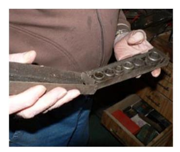
A set of box spanners that Dad bought in 1924 to go with the T-Model Ford that he bought then to run the butcher's cart. They're all SAE Standard.
