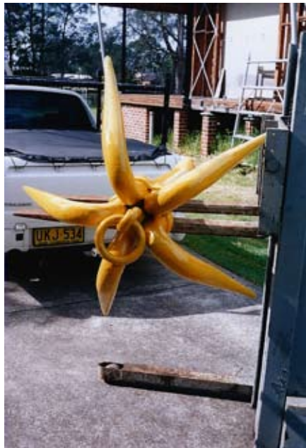
This is the grapple we use for anchor recovery
